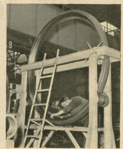
This is a job for a very steady hand. An expert files the scores of cogs on a Centurion turret ring, which is held in position by a giant clamp.
