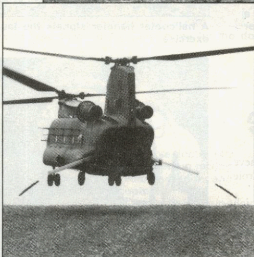
Above – As the Chinook mine layer flies on, two sappers arm the lethal bar mines. The technique was developed by 51 Field Squadron RE
