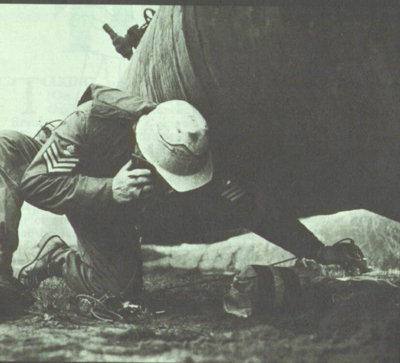
Using a stethoscope on a bomb under a fuel pipe at an oil refinery. Below: Portable X-ray equipment used by WO II Norman Humphries.
