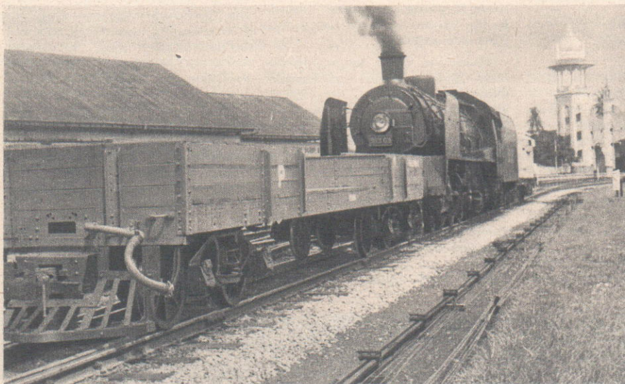
In front of the engine of the pilot train is a low truck loaded with iron bars to assimilate the shock of a mine. Right: The locomotive cab with steel doors closed.
