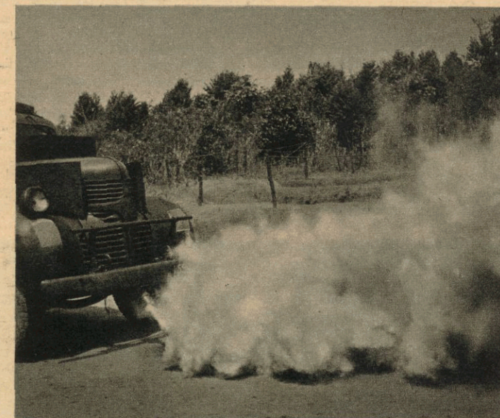
For the lorry-driver, making this smoke-screen is as simple as switching on his headlights. The smoke-generator is connected with the lorry's battery.
