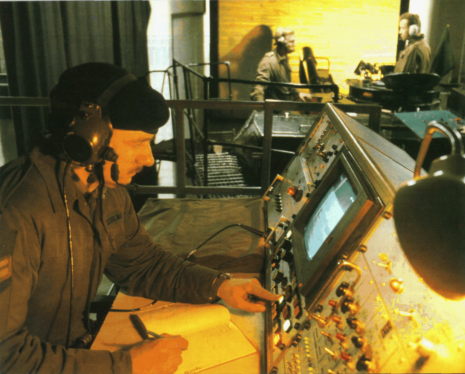
From his control console, a gunnery instructor analyses the performance of a tank crew on the Gunnery Training System (GTS). An improvement in gunnery standards has been attributed to the system
