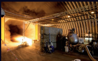
FLAMING FORCE: BLOODHOUND'S HYBRID ROCKET PRODUCED 14,000LBS OF THRUST
