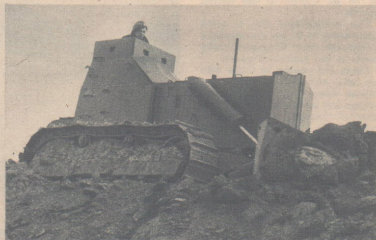
Bulldozers may have to operate under fire, hence the armour-plating on this one.
