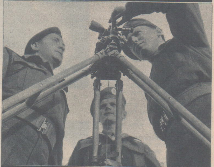
Above: You want to know where to make a curve in a road? Students in the Survey School will use a theodolite to measure the place up and let you know. Below: You want to know how thick to make a road surface? Quartermaster-Serjeant Instructor D. J. Johnson of the Soils Laboratory is finding out with the help of a piece of earth and a few chemicals.
