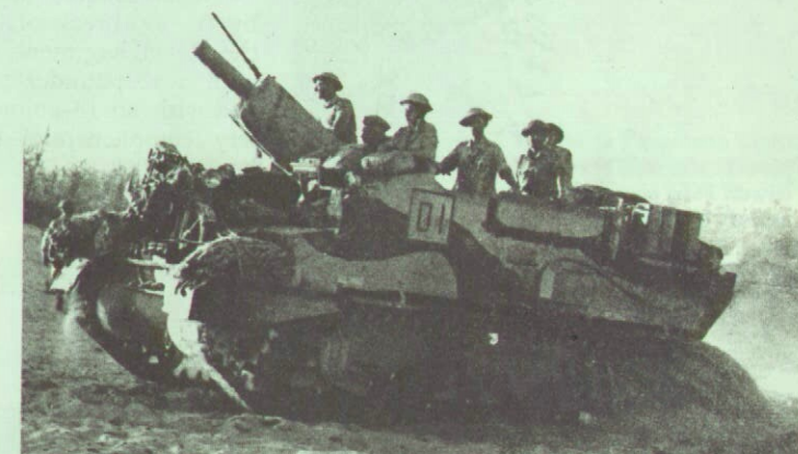
Bishop (25-pounder, Valentine) gave way to Priest (105-mm howitzer on Grant, later Sherman chassis), seen here on beach in invasion of Italy.
