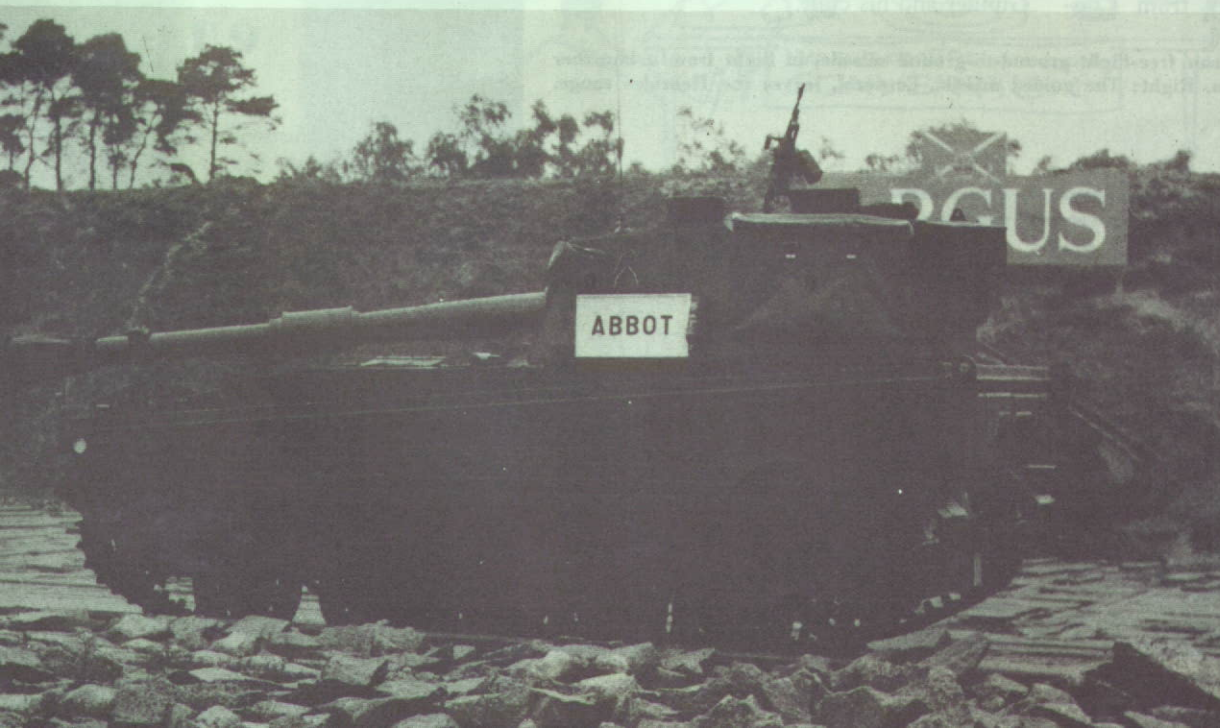
Left: The self-propelled British 105-mm Abbot, another current equipment, can traverse 360 degrees.
