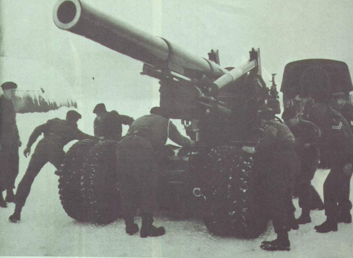
The United States 8-inch howitzer, on the British 7.2-inch mounting, fires a nuclear or an HE shell.
