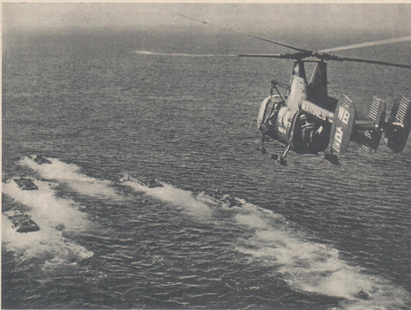
Another role for the versatile helicopter: guiding amphibious vehicles by remote control. This picture, taken on the Californian coast, shows a HOK helicopter steering unmanned landing craft ashore. The "driver" is a passenger in the helicopter who operates an electronic control panel which starts and stops the landing crafts' engines, changes gear, steers, brakes and applies the throttle.
