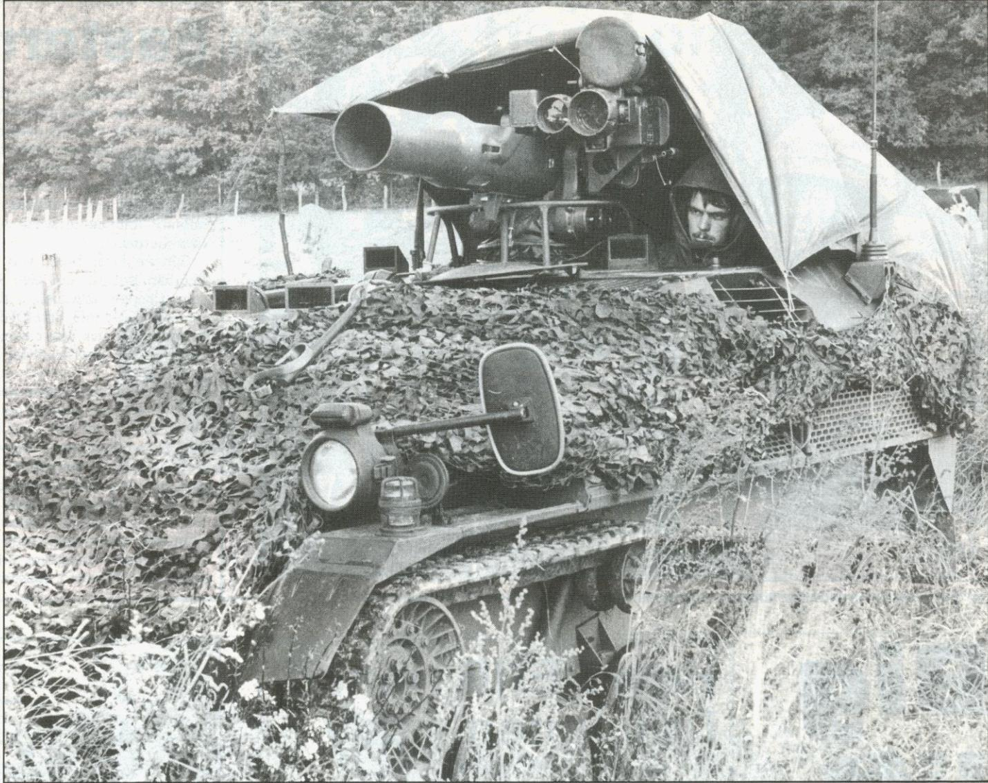
Wiesel with TOW - small and easy to conceal. Designed by Porsche, it is a nippy mover and its tracks are made of rubber
