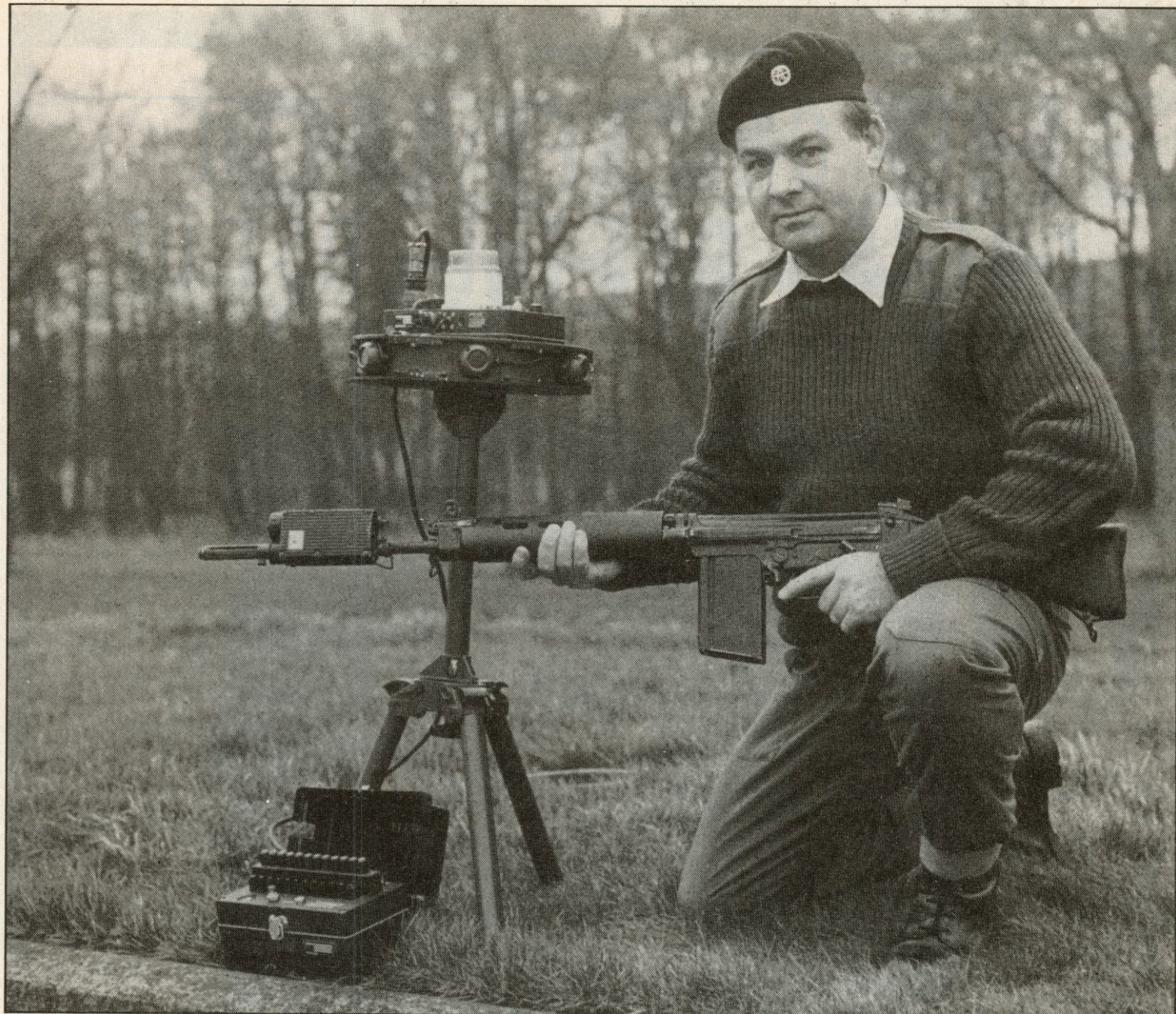
WO1 (TSM) Warren Larnder shows off a weapons effects simulator rifle and a remote laser-controlled exploder system
