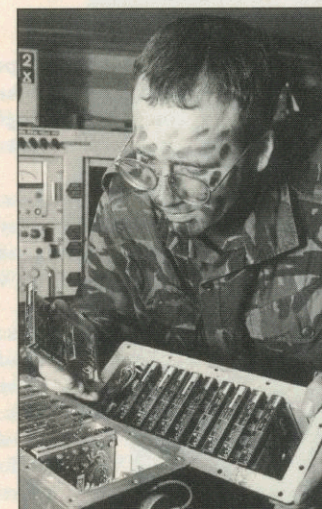
Above: Sgt Ash Houghton REME tests Rapier's amplifier electronic control in the electronic repair vehicle of A2 echelon
