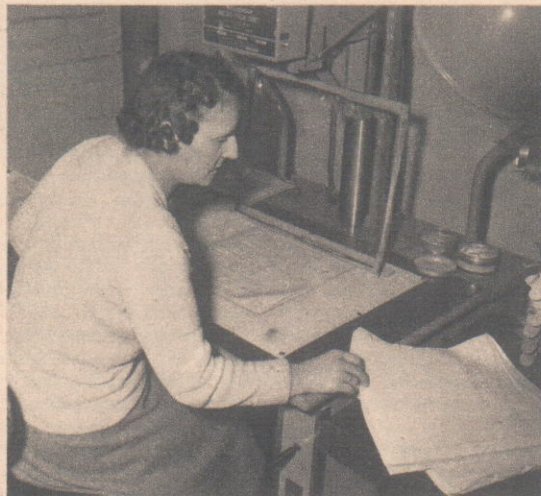
At the micro-film camera: the operator in this picture is photographing soldiers' records of service. The actual camera is above the operator's head. Below: On the left a film is drying. On the right is the "reader" on which films are checked before they are sent off.
