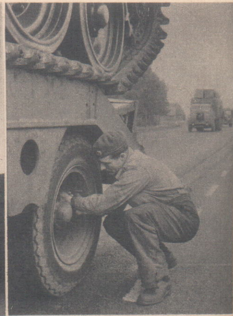
Testing tyre pressures: on the road, the driver examines each tyre every two hours.
