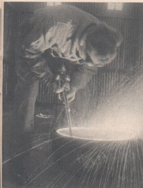
Bowl of fire. A hub casing is repaired in the company's workshop.
