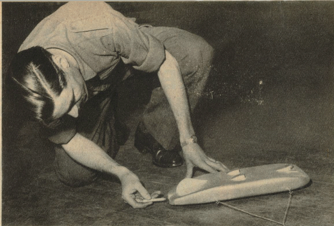
A lighted cigarette-end is all that is needed to start SQMS R. Eade's jet-propelled "Railton." The engine is powered by solid fuel capsules.
