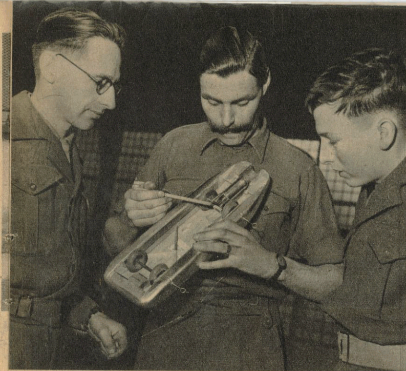
The designer shows how the jet engine is fitted in his racing car. It has a thrust of four-and-a-half ounces.
