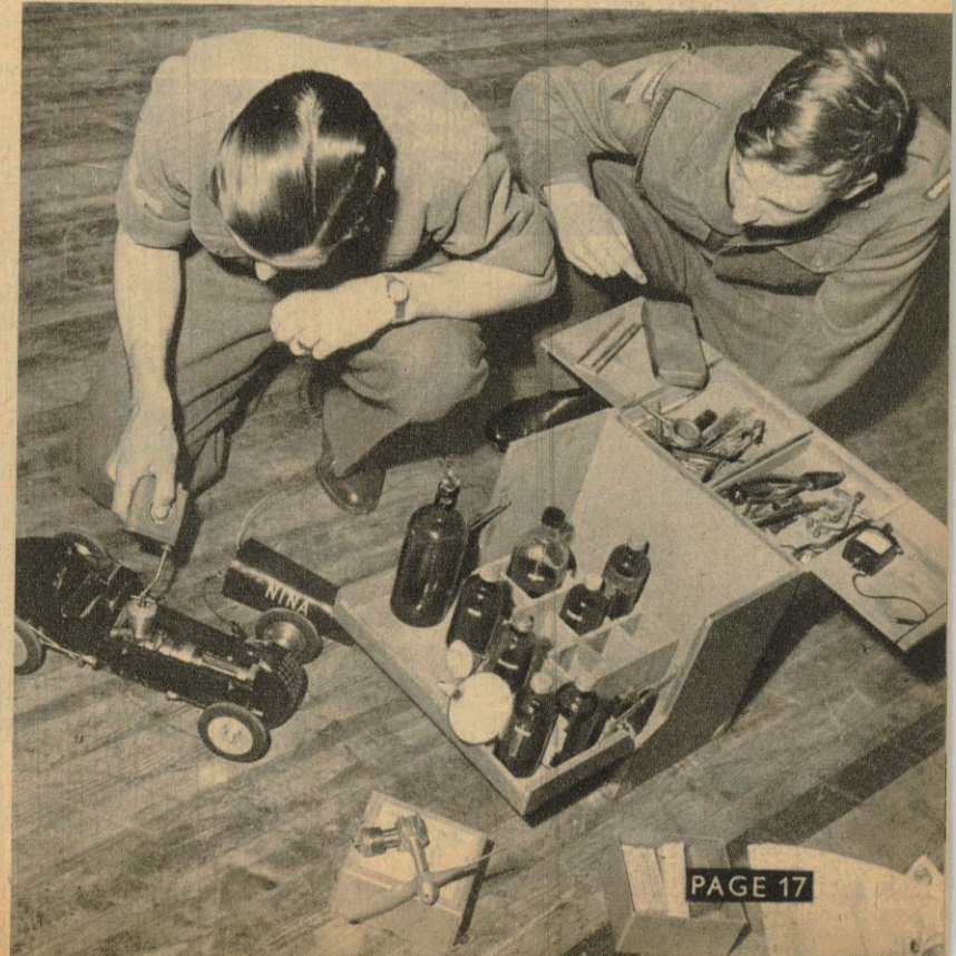
It's easier to start the engine of a model aircraft with this "home-made" machine, driven by two old accumulators. Otherwise you have to turn the propeller by hand.
