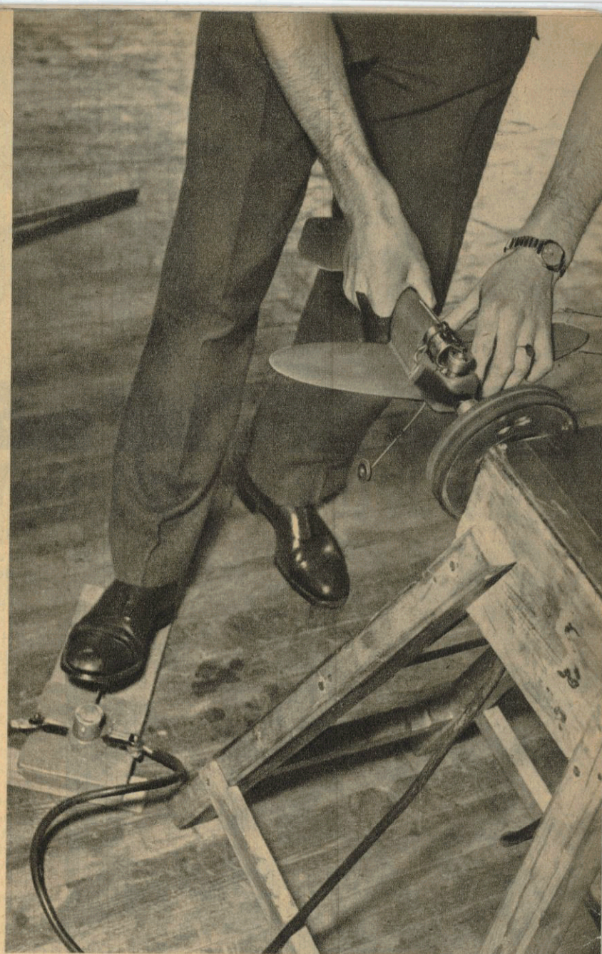
It's easier to start the engine of a model aircraft with this "home-made" machine, driven by two old accumulators. Otherwise you have to turn the propeller by hand.
