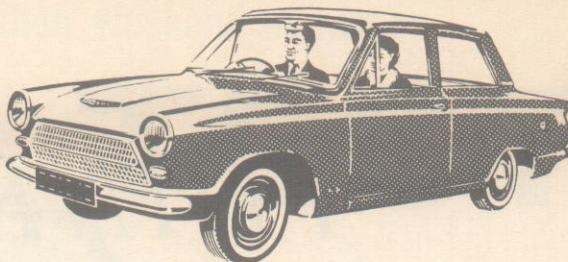
From Ford comes a new Cortina with a power of difference—the outstanding new Cortina G.T. The power isn't the only difference. To terrific performance Ford have added luxury and enviable finesse. 0-60 in 13.2 sec. Top speed 92 m.p.h. 1500 c.c. engine. Remote gear shift. Raised compression ratio (9.1). Modified combustion chamber. Larger exhaust valves. Weber carburettor and air cleaner. Free flow 4 branch exhaust manifold. Modified camshaft. Front disc brakes.
