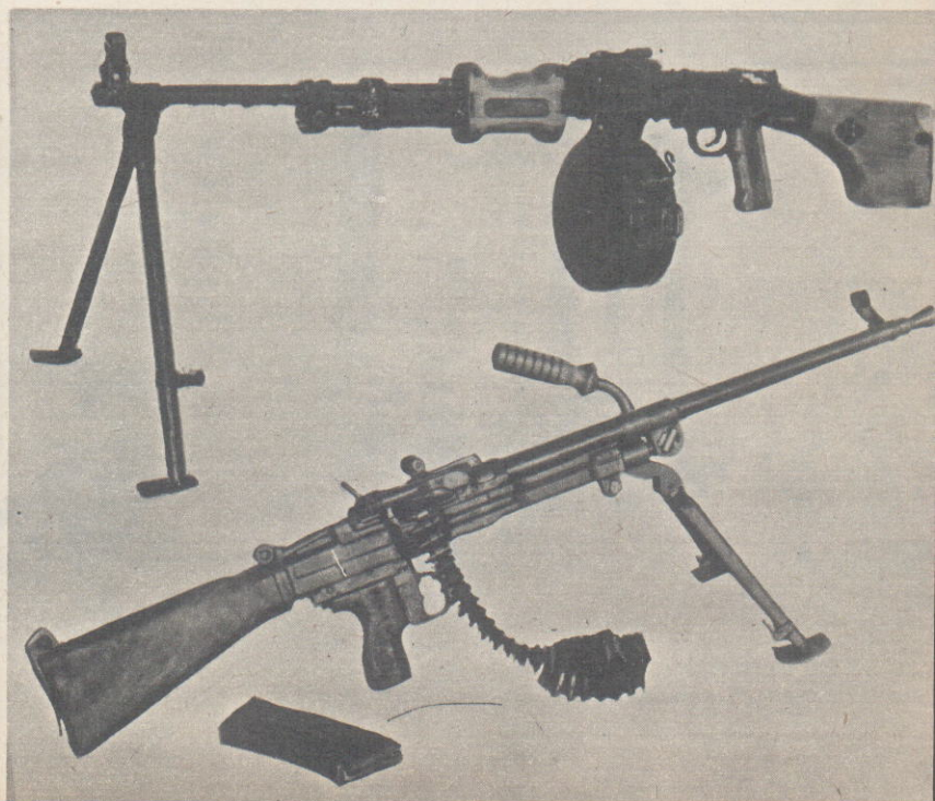
Parachute troops pose on a captured tank. Right: British soldiers captured these light machine-guns in Egypt. They are (top) a Russian 7.62 mm, fitted with a magazine containing 100 rounds and (below) a Czech 7.62 mm, made by the BRNO factory that produced the Bren. This unusual weapon is fed by magazine or belt.
