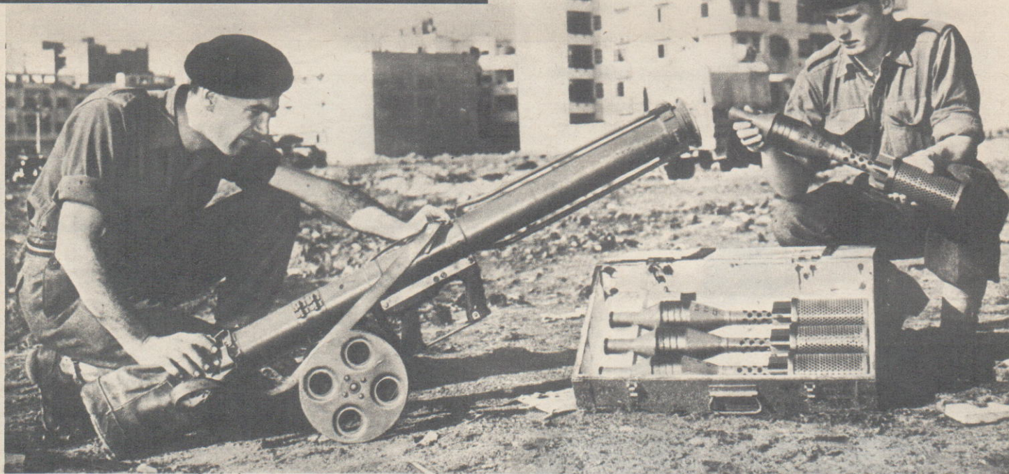
A Czech recoilless rocket launcher used by Egyptian Infantry is examined by Pte. Kenneth Yoxall (left) and Cpl. Peter Absalom. This smooth-bore, 82 mm anti-tank gun is fitted with wheels so that it can be towed by hand.
