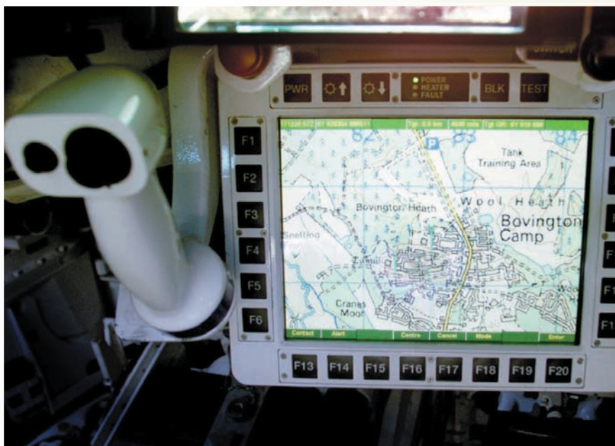
Testing time: The P Bisa system in the commander's crew station of Challenger 2
