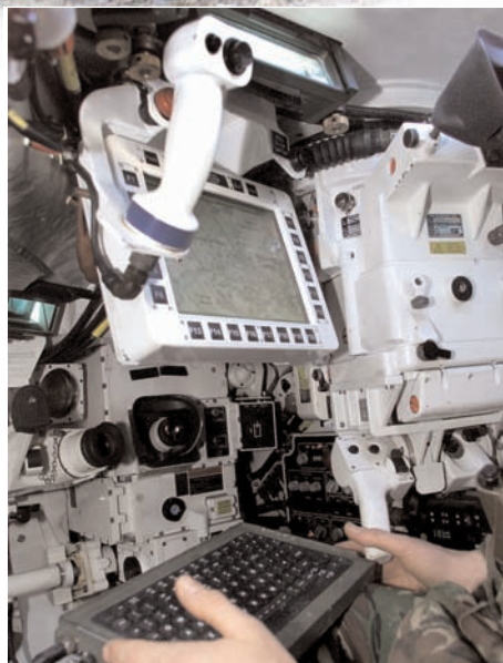
Getting the point: The P Bisa system display in Challenger 2 includes a pointing device
