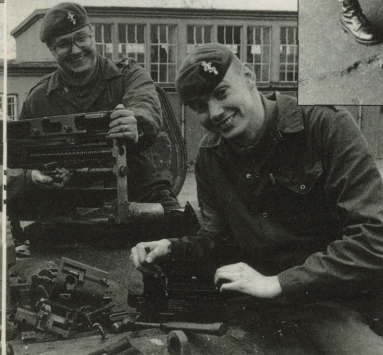
Below – Chain gang: Cpl Tommo Thomson and Cfn Phil Mills of the armoury shop work on the top casing of a cannon, while LCpl 'Washy' Washbourne tackles the main body of a chain drive from a chain gun
