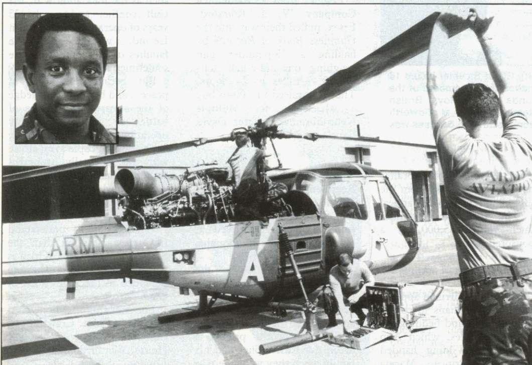
Sgt John Broughton checks a droop stop ring while Cpl Nick Bird selects a tool and Cpl Mark Stainthorpe lifts the blade of a Scout undergoing maintenance at Borneo Lines
