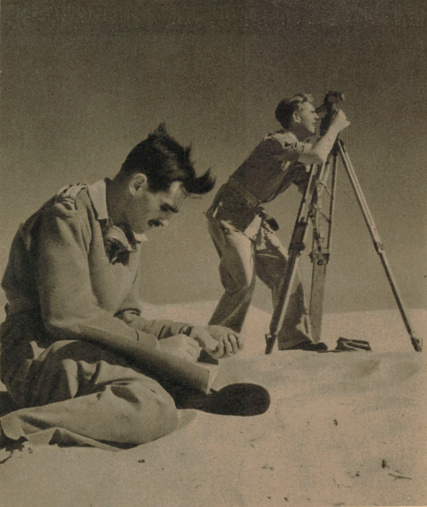
While Captain A. L. King-Harman takes his theodolite reading on the stars, Captain C. S. Wallis-King checks the reading times with a stop watch.
