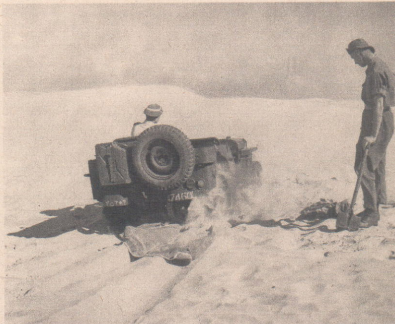
When the jeep wheels sink, the sand must be dug away and a tarpaulin "fed" underneath so that the treads can grip.
