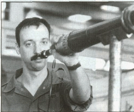
Cpl Ray Smith checks the bore of Rarden cannon barrel, main armament of the Light Dragoons' Scimitars
