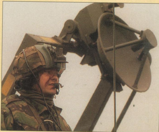
Virtual reality: Operators wear a sophisticated electronic helmet sighting system. Where Sgt Philip Yee looks, the Rapier's radar dish follows
