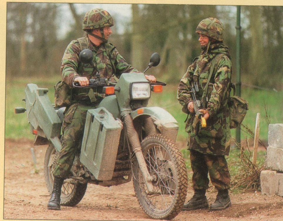
Exercise despatches: Sgt Steve Stewart with one of the Harley Davidson motor cycles that have just entered British Army service. Gnr Mel Byren discusses its merits. The pannier mounted on the rear is designed for weapon stowage. An SA80 fits easily into the compartment
