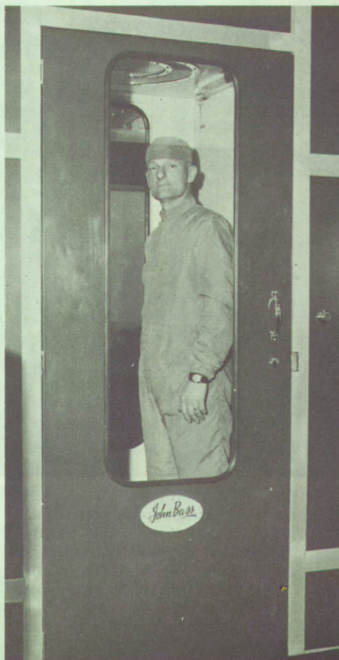
The inner sanctum of the Clean Room is reached only through this air lock inside which the men are cleaned by air jets before entering.
