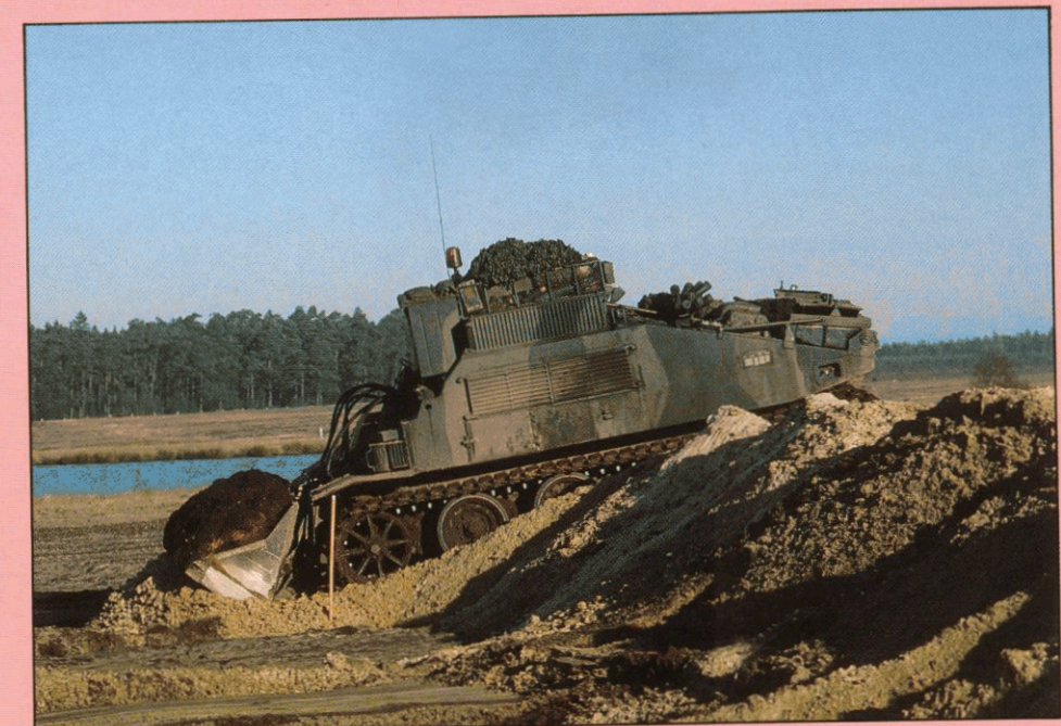
A Combat Engineer Tractor (CET) advances with its bucket already full of earth which it can dump immediately into any crater
