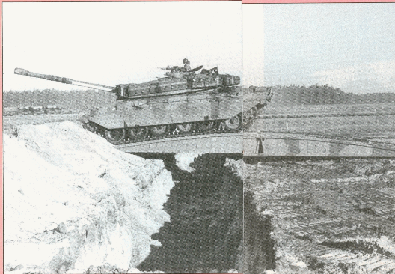
A Challenger tank of 14/20 H crosses a ditch using a No 9 tank bridge
