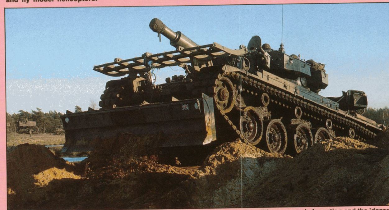
A Centurion AVRE, having dropped its fascine, advances with the 165mm demolition gun ready for action and the 'dozer ready for work
