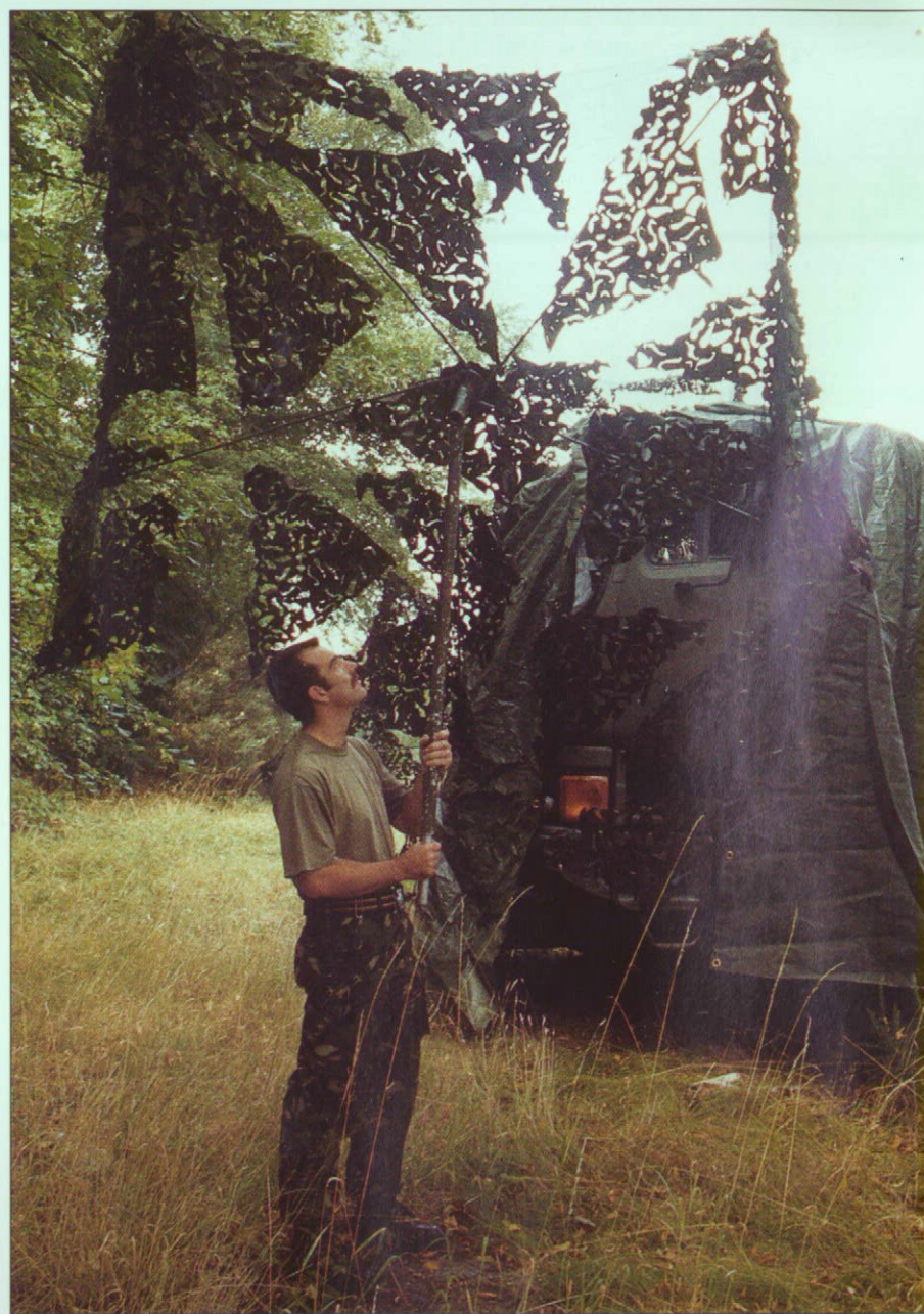
Now you see it: The "cambrella" umbrella camouflage system which the Trials and Development team claims can be erected much more rapidly than conventional camouflage netting
