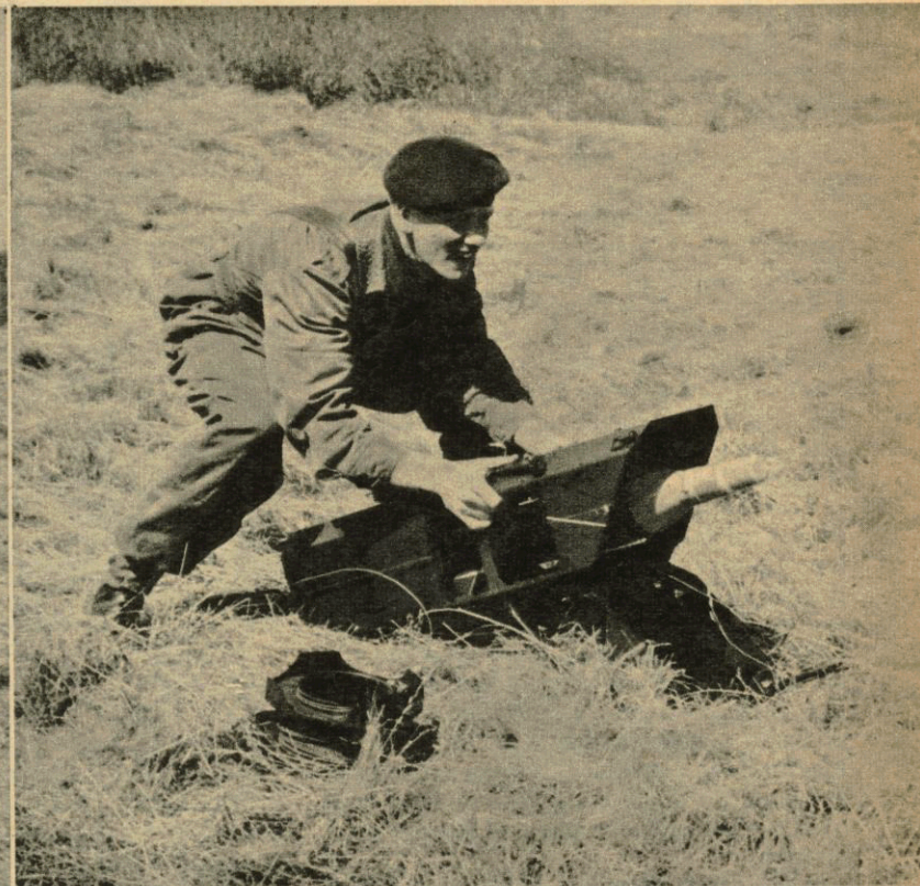
2 No pre-assembly is required—the launcher-box is simply positioned at an angle of 30 degrees to the ground facing the target.
