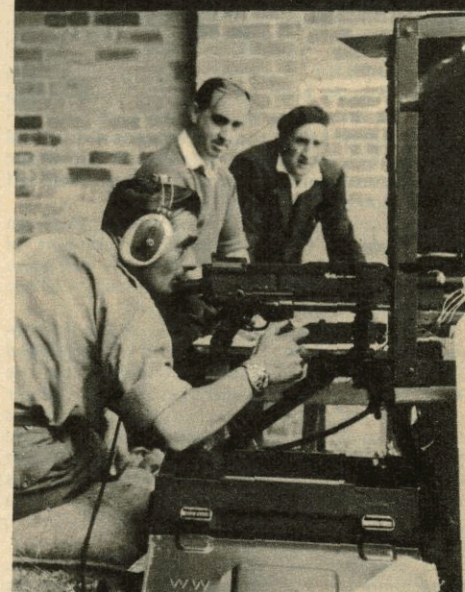
Above: The 7.62mm General Purpose Machine-Gun is put through its paces for barrel wear, accuracy, velocity and rate of fire.
