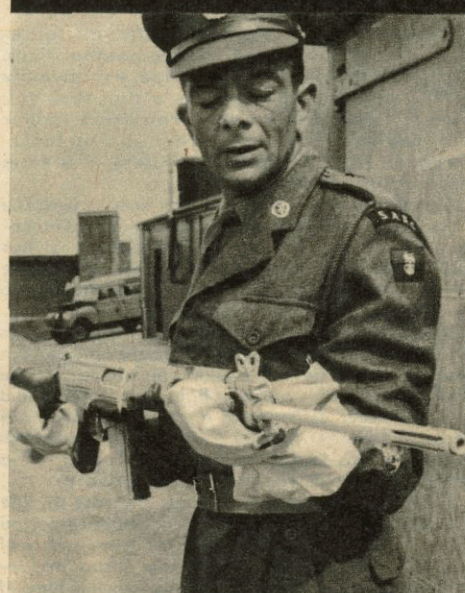
Wearing protective gloves, EQMSI R. Dickens inspects a frost-covered automatic rifle after its removal from the cold chamber.
