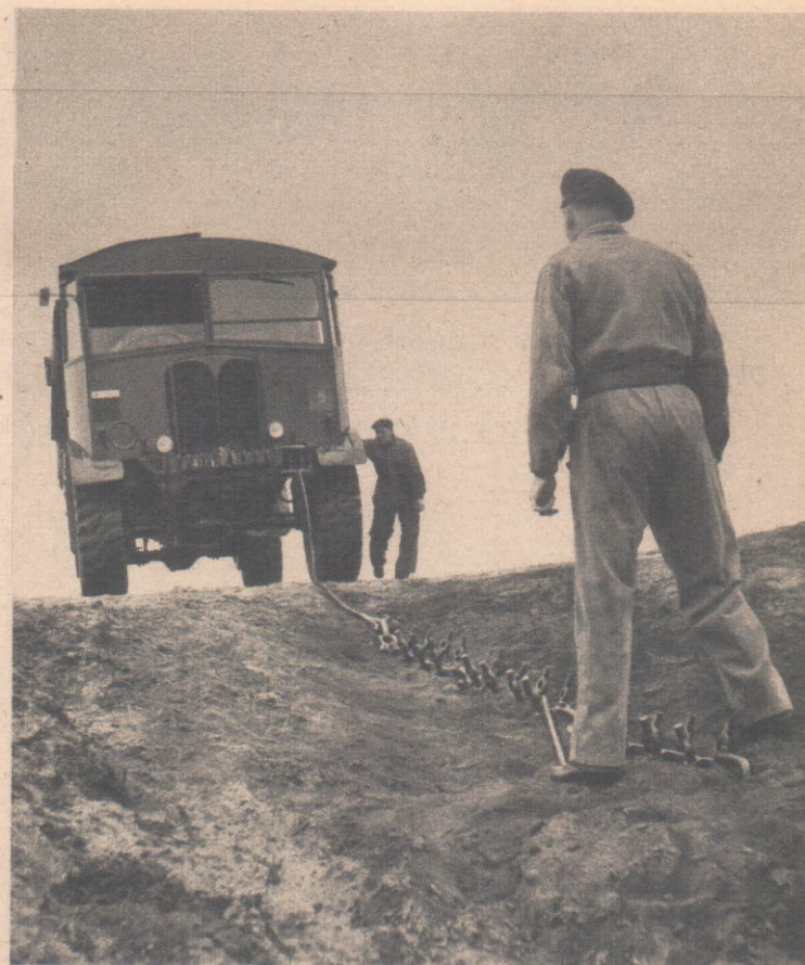
A Matador winches itself up a gradient of one in two (left) to its ground anchor (above). Once at the top, it will winch up the gun it was towing.
