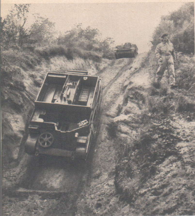
A trick for special occasions. The track is suspected of being mined, but the driver is in a hurry. So he sets his carrier in low gear and walks behind. Steep banks will keep the carrier from straying.
