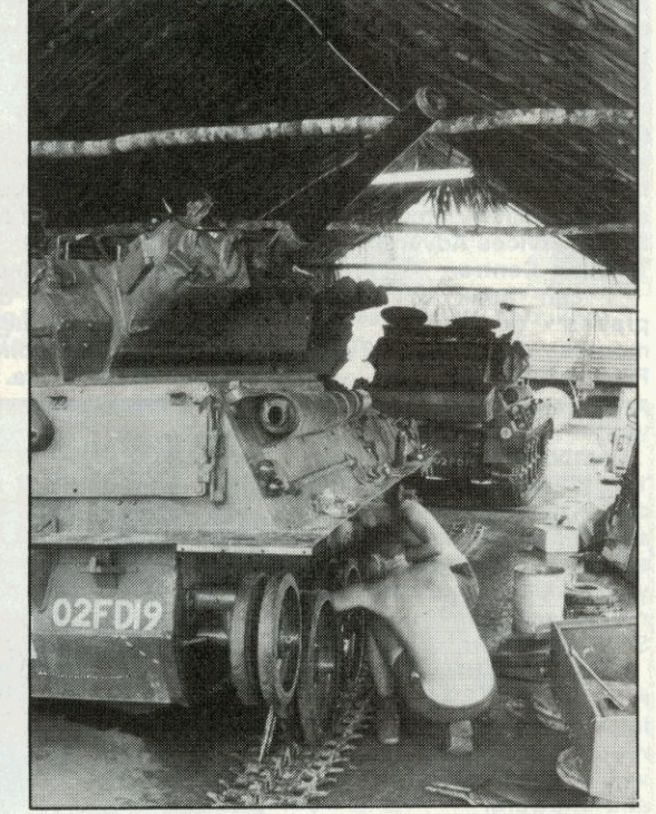
REME mechanics attached to the Scots DG strip a Scorpion under cover
