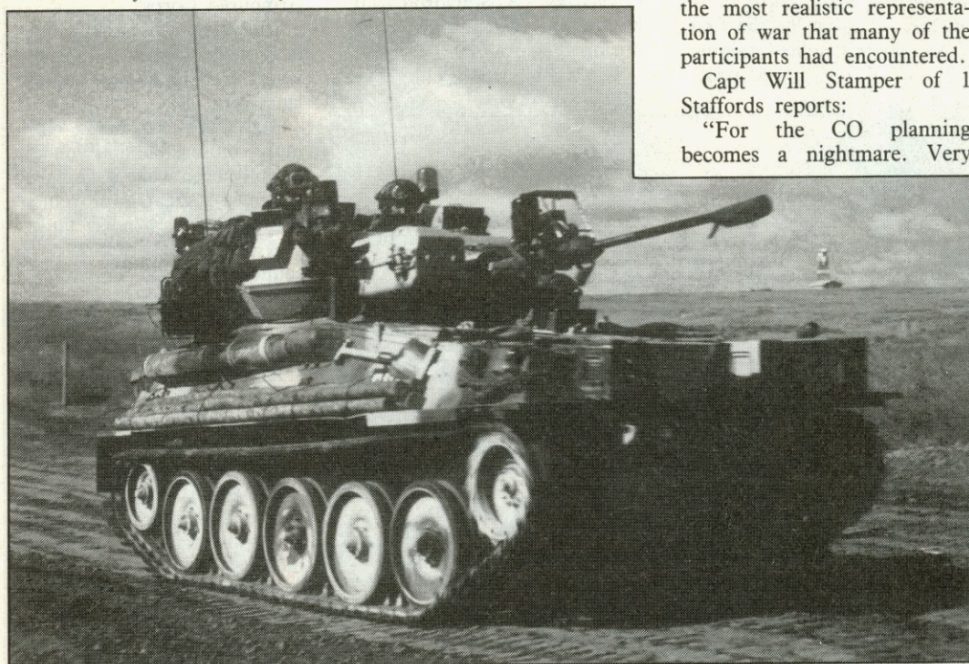
A Scimitar from the recce platoon of 1 Staffords deploys in BATUS. A rear light flashes orange to indicate the vehicle has been hit while a red light mounted on the main armament indicates when the Scimitar is firing
