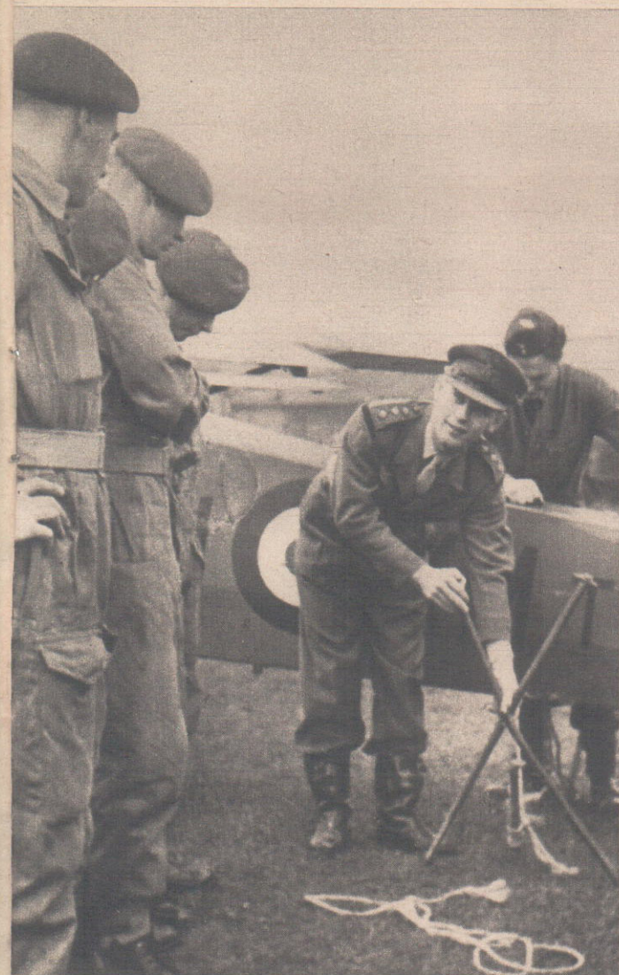
Left: In stormy weather an Auster must be tethered to the ground. Here students learn how to set out pickets.
