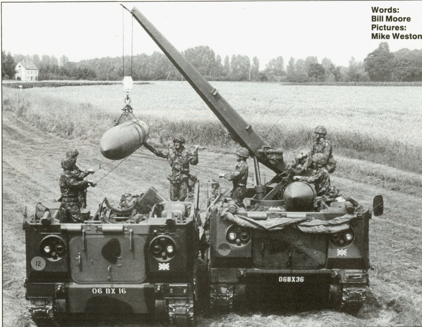
Missile re-supply in the field. Launcher left, loader transporter right
