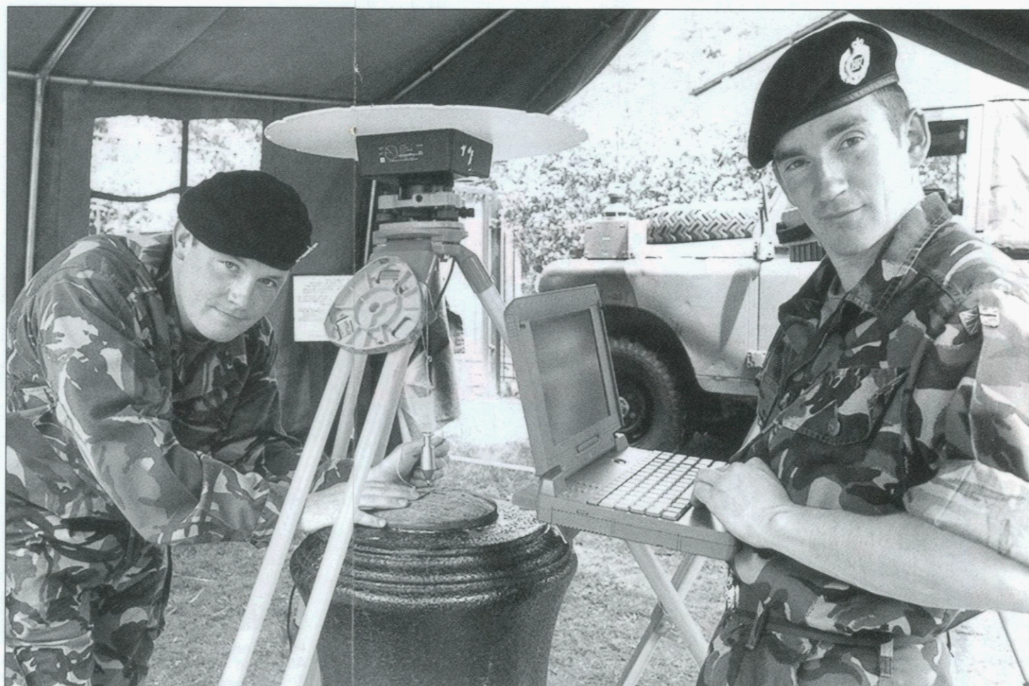
Sgt Andy Gray and Cpl John Leighton check the data from the Trimble 4000 SSE Survey Grid GPS receiver over the cannon head in Hounslow
