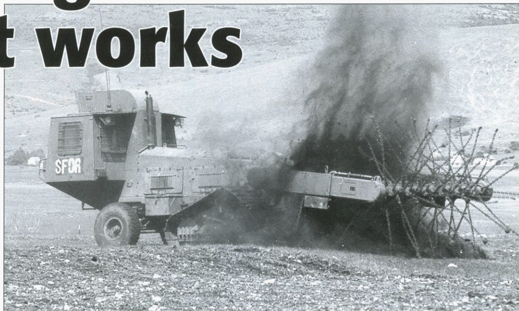
Aardvark, the British Army's mine clearance vehicle, raises the dust in Bosnia
