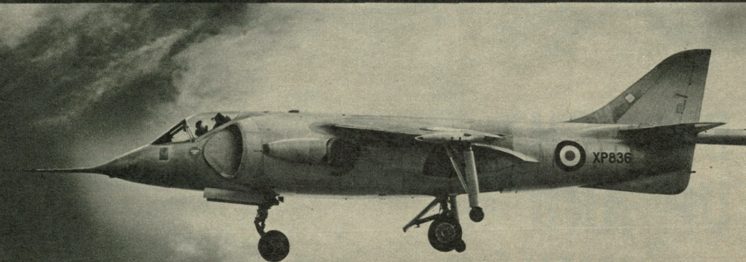
The P.1127 in flight. This aircraft, now undergoing Government trials, can operate as a strike fighter, armed with rockets, or a recce plane.
