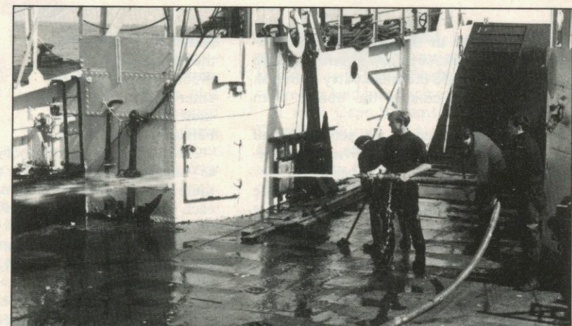
Landing craft crew hose down the deck after dumping in Beaufort Dyke. All traces of explosive and inflammable material have to be washed away
