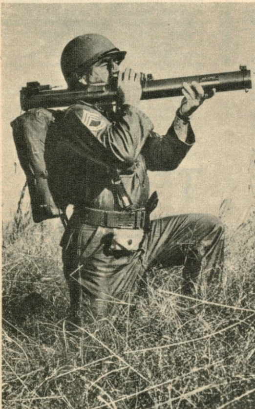
New, too, is the US Army's anti-tank rocket grenade, fired from its own disposable packet container. Highly effective against tanks, light fortifications and armoured vehicles, it can be carried and fired by one man.
