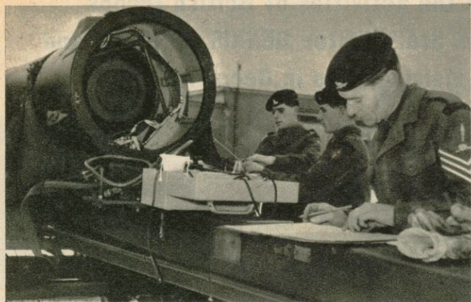
At the rocket's business end, before the fins are fitted, Sergeant C. Saddington, RA, checks the assembly on a pole trailer. In this process all electric parts and circuits are tested and carefully re-checked.
