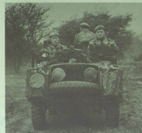
A design for the standard SAS Land Rover close to the finally approved version. In the end the unit produced its own blueprint for adaption to the raiding role.
