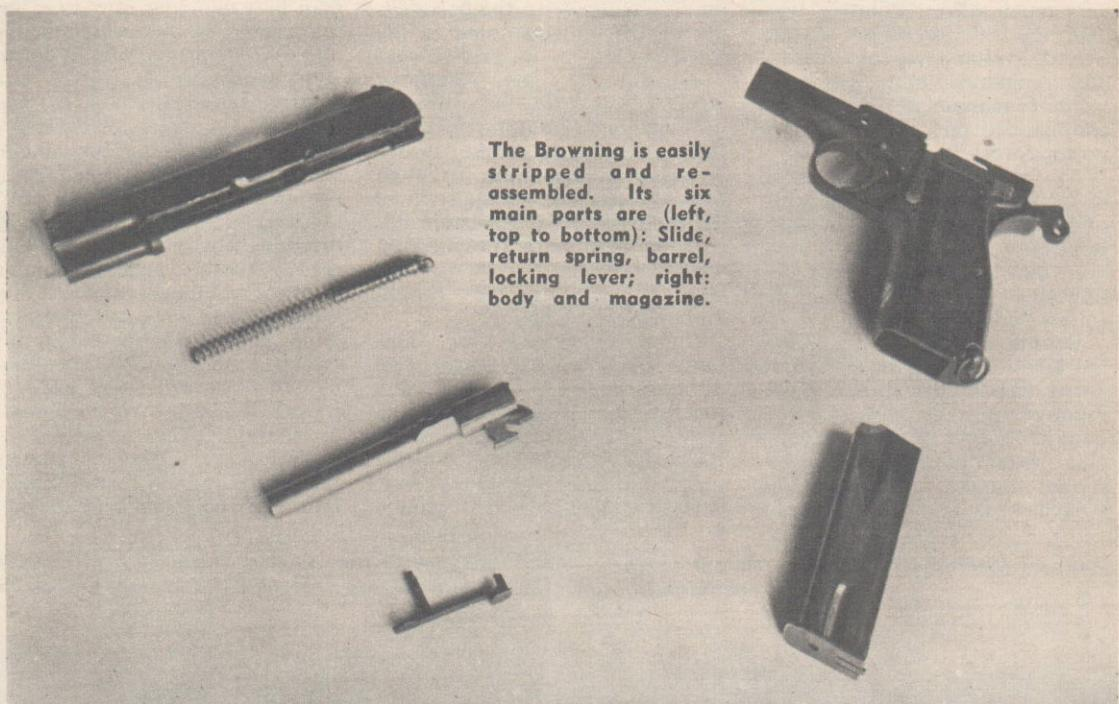
The Browning is easily stripped and reassembled. Its six main parts are (left, top to bottom): Slide, return spring, barrel, locking lever; right: body and magazine.
