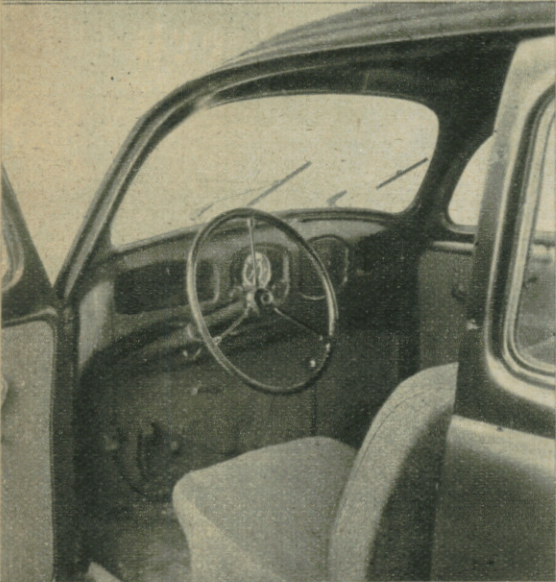
View of the driver's seat and controls. The lay-out is neat but not skimped, and there is plenty of leg room, as the engine is in the rear.
