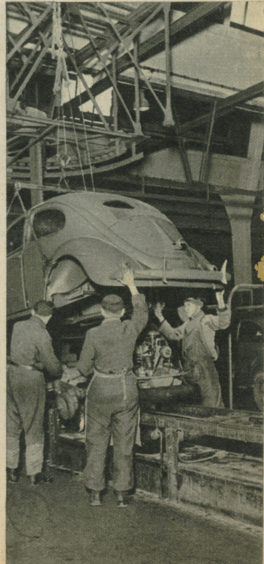
Below: Final assembly line: fitting the all-steel body on the chassis.
