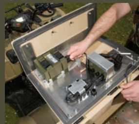
A charging unit fitted in the trunk of a quad bike provides added energy for a patrol's batteries
