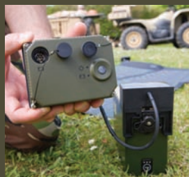
The Soldier Portable Charger unit gives troops on patrol a mobile source of power generation
