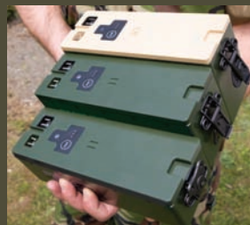
LIPS 10 - Bat life: Six hrs - Wt: 3.75kg LIPS 11 - Bat life: Two hrs - Wt: 1.5kg LIPS 12 - Bat life: Four hrs - Wt: 2.25kg
