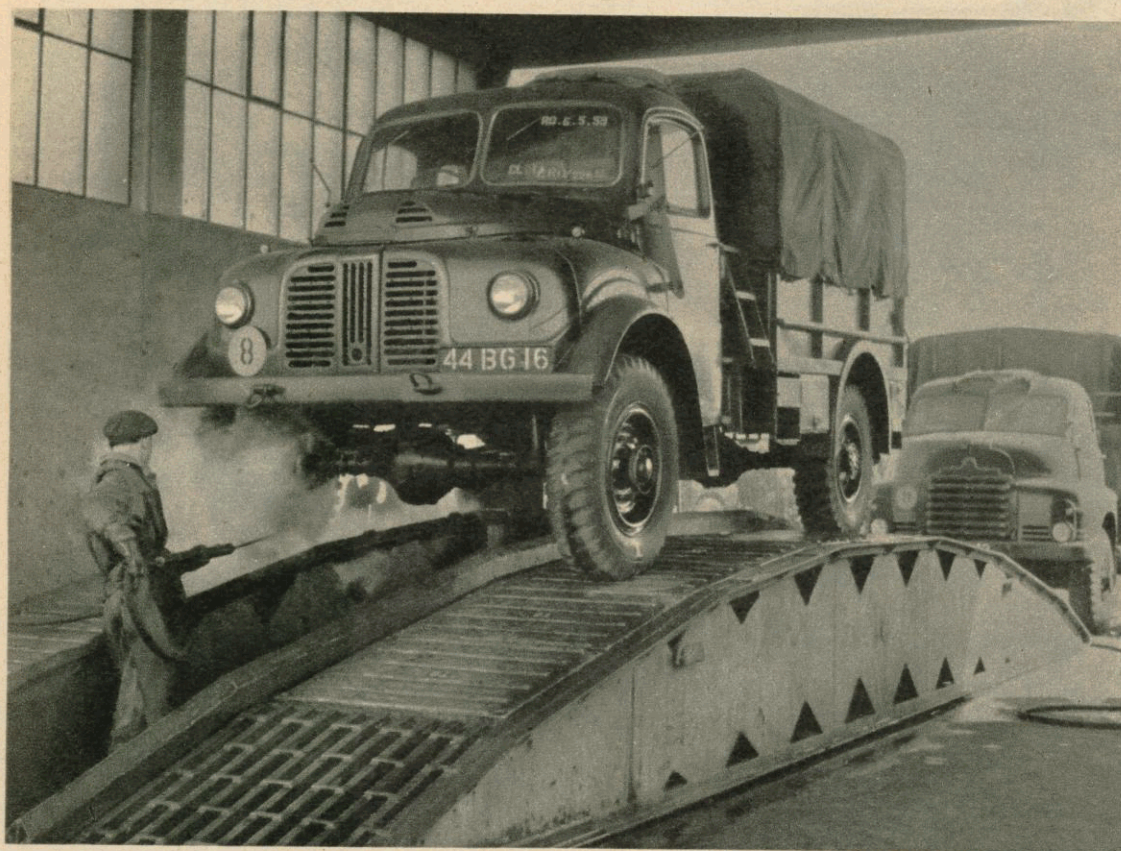
Above: The powerful jet of a steam jenny whips away dust and grease as a three-tonner from store is cleaned ready for issuing to a unit.
