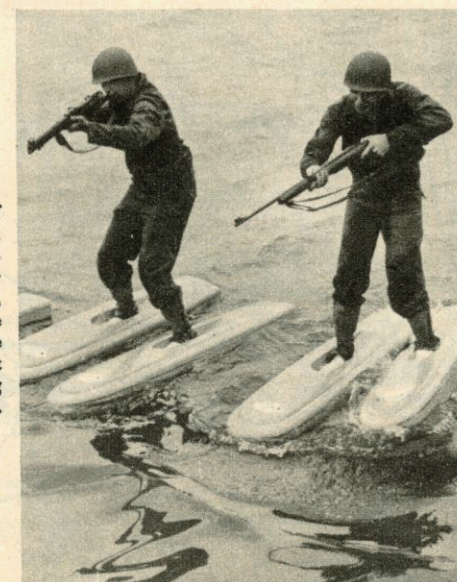
United States soldiers demonstrate a military form of water-skiing. The rigid foam water shoes enable them to walk at three miles an hour over rivers, lakes or swamps, with both hands free to fire their rifles. The shoes can be lashed together to form a raft on which a soldier can drag a casualty or supplies.
