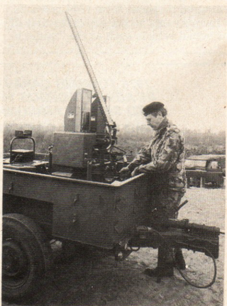
Below: MIDGE homing beacon which sends out a signal to bring it down.
