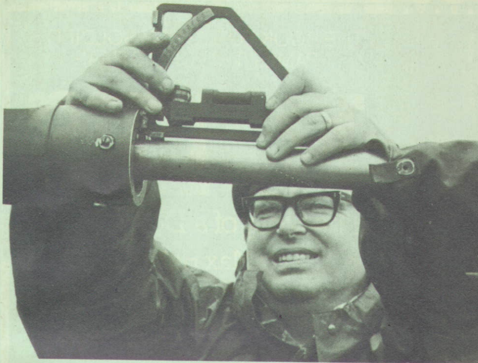
◀ Using an inclinometer to make sure gun's alignment is correct.
