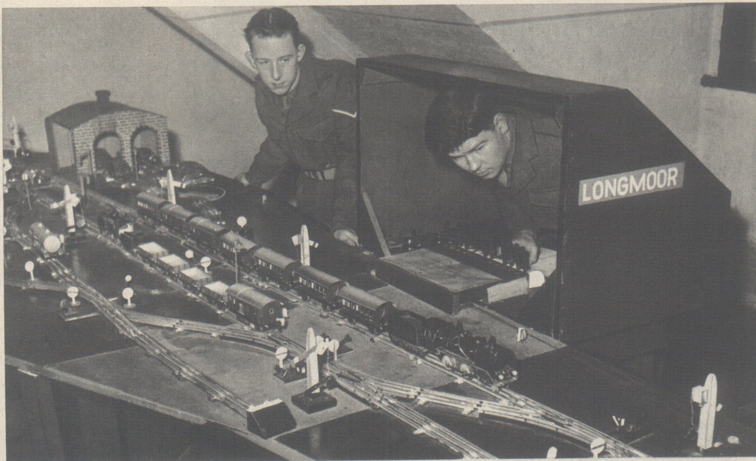
On this model railway Lance-Corporal I. H. Rogers watches Sapper F. J. Butler, a block-man, pass a passenger train from a siding on to the main line.
