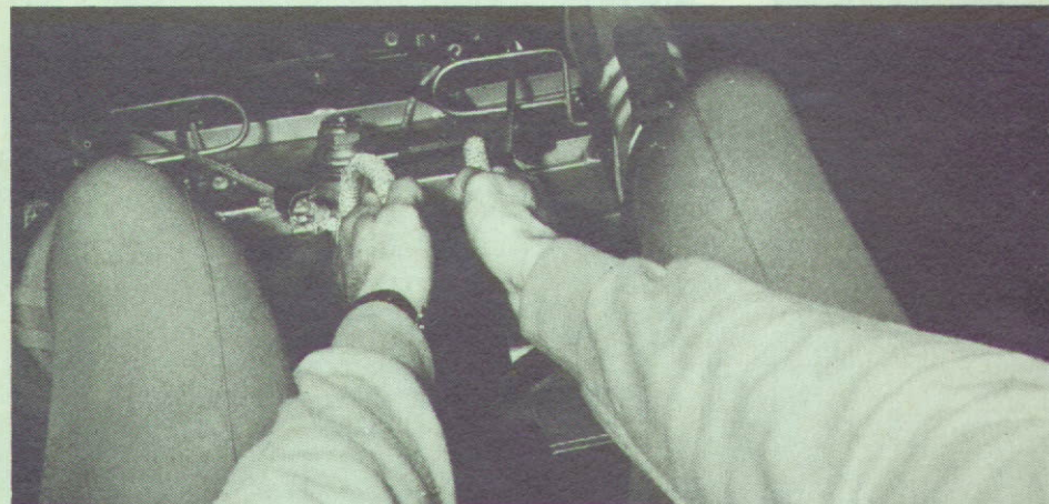
Above: Inside the bobsleigh — a driver's eye view of steering reins and foot controls.
