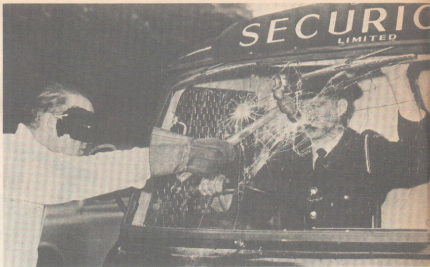
Above: Special toughened glass is just one of the safety devices included on the armoured vehicles.
