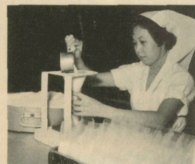
With measuring scoop and fixed funnel, sugar is bagged simply and speedily.
