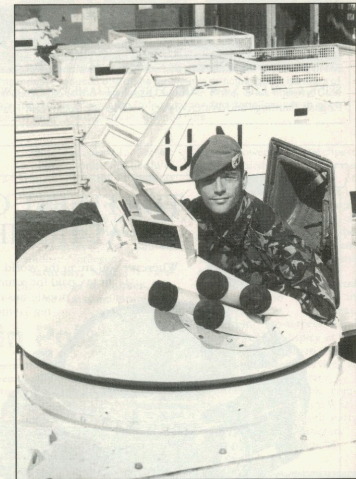
A snug fit! Pte Anthony Simpson, 1 DWR tries out the first L37 turret fitted to Saxon in Bosnia. Note the angled wire-cutting device in front of his hatch and the smoke dischargers
