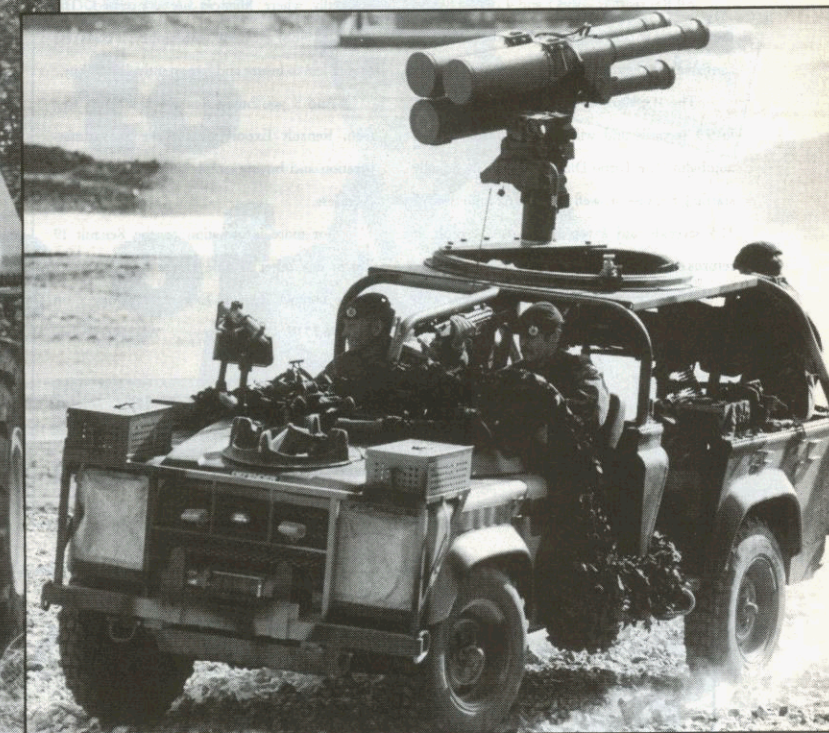
Above – Airborne sappers demonstrate Land Rover's special operations vehicle fitted with Starburst laser-guided close air defence missile system
