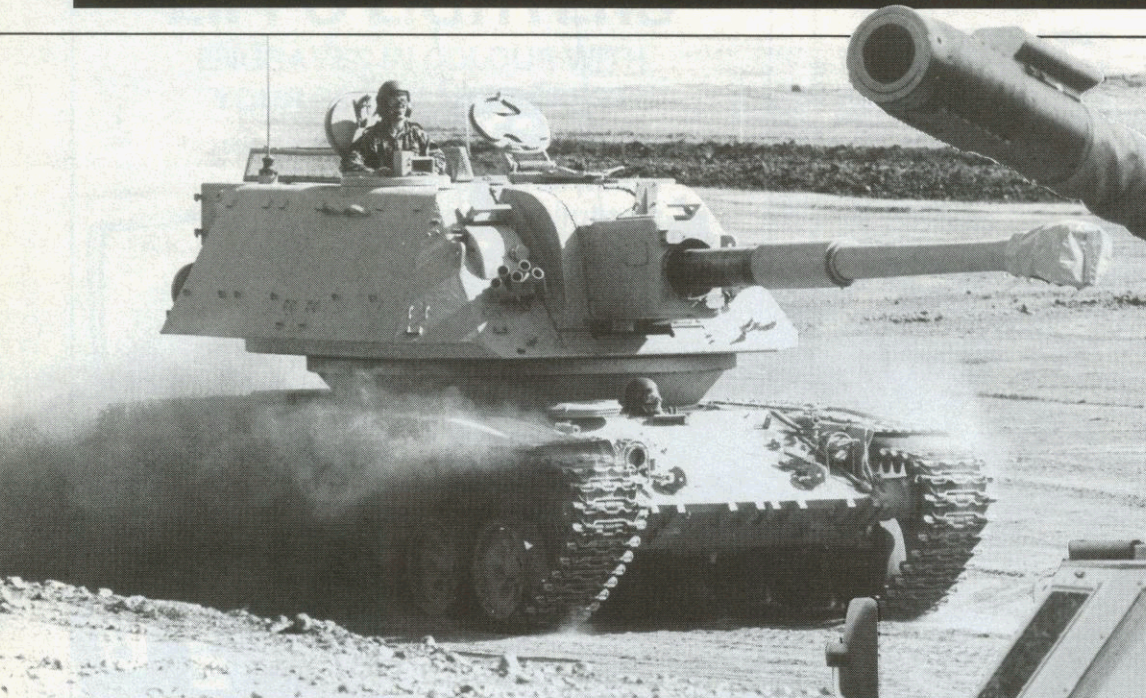
Strangest-looking vehicle on display was this Russian T-72 main battle tank chassis fitted with the AS 90 155mm self-propelled artillery system
