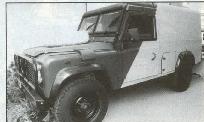
Two-tone CAV100 light armoured vehicle part-painted with the new quick-change camouflage paint
