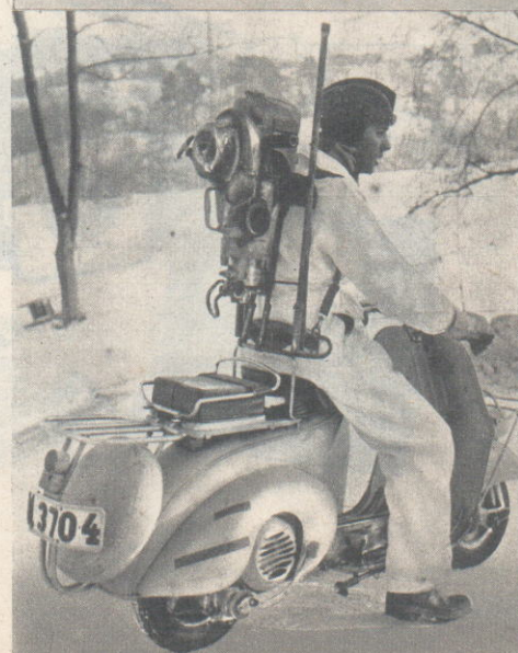
The Cobra in action on a thick block of reinforced concrete. It can drill through rock at more than six inches a minute and is useful for enlarging trenches. Below: The Cobra is a one-man load, weighing only 53 lbs.
