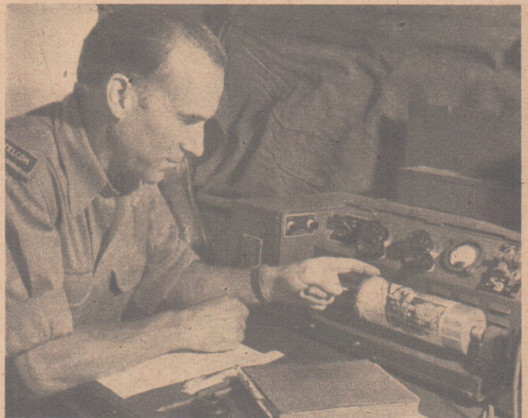
The picture on the drum is being radioed to London.
