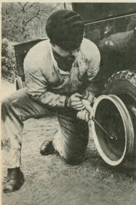
A REME craftsman tightens the nuts which hold the flanged hubs to the wheels. The hard steel cable bites into the soft metal hubs and allows the vehicle to drive across under its own power.
